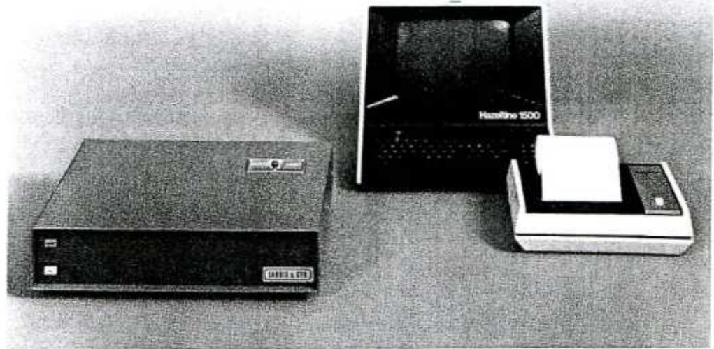
Fig. 6 ID 2000 card programming unit with display terminal and printer.
